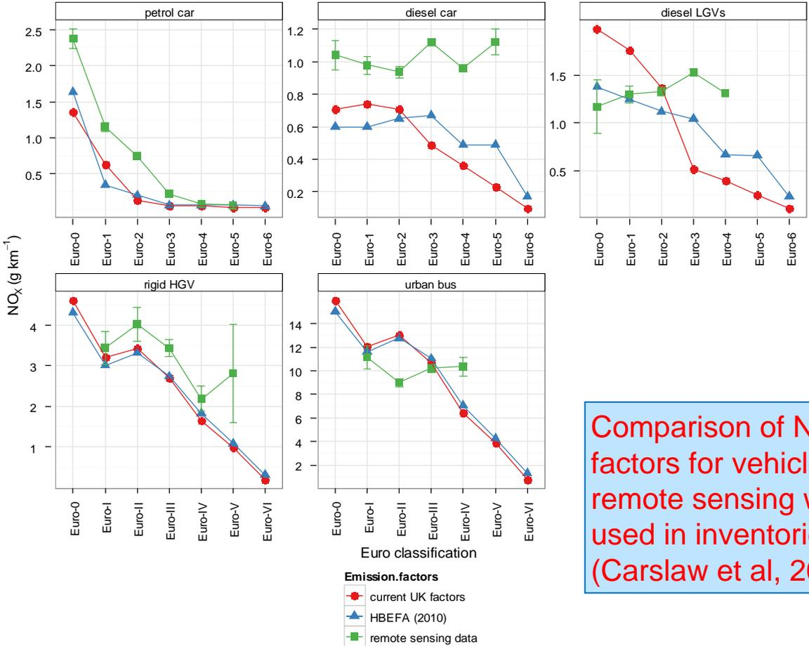
Comparison of NO<sub>x</sub> emission factors for vehicles derived from remote sensing with factors used in inventories (Carslaw et al, 2011)
