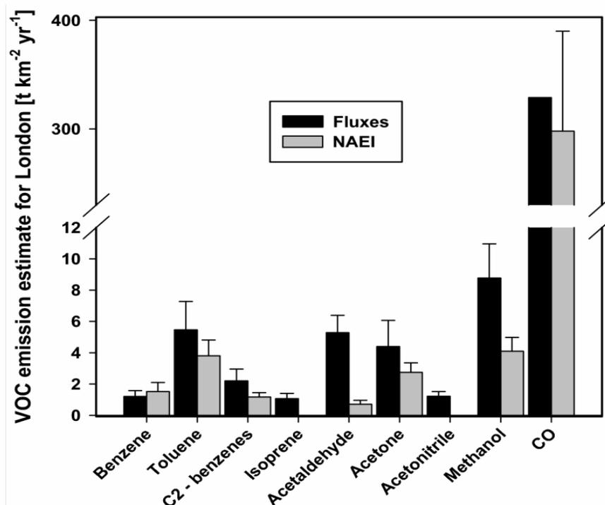
Comparison between NAEI estimates of emissions and those derived from flux measurements over London (Langford et al, 2010)
