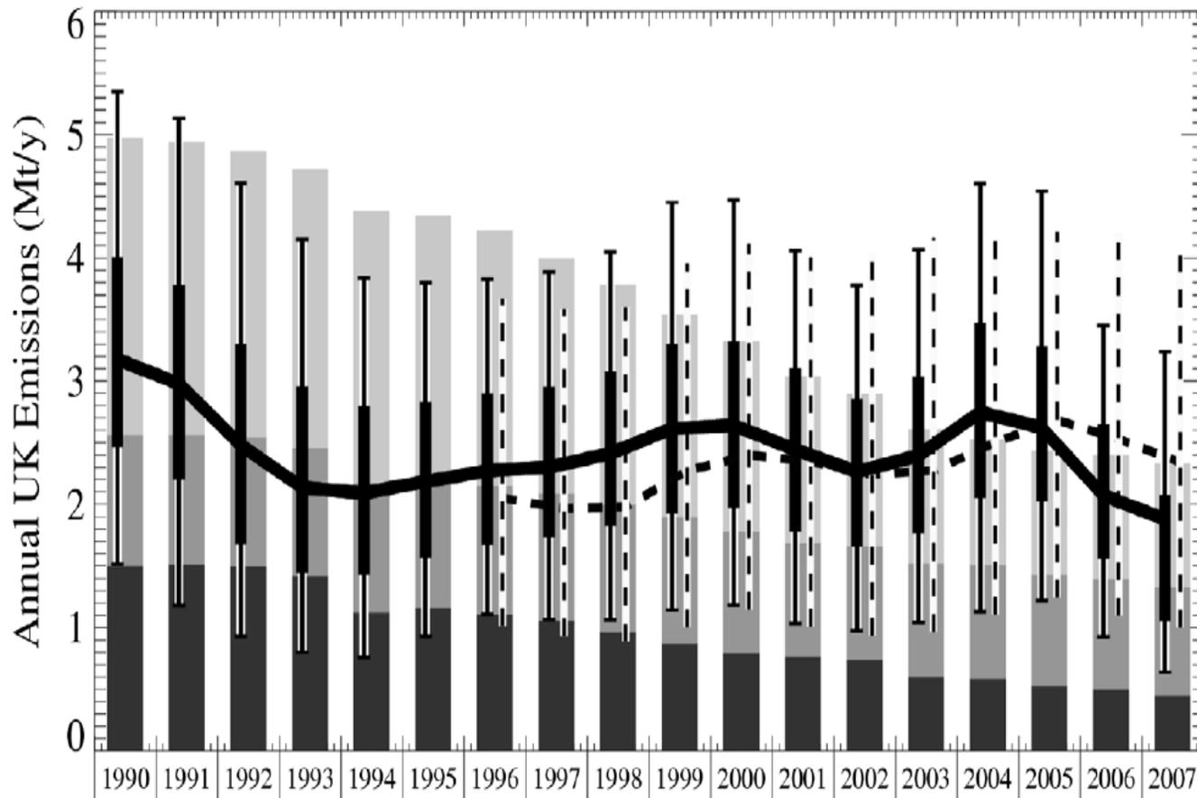
UK emission estimates for CH<sub>4</sub> based on NAME inversion (line) and UK GHG inventory. Cumulative columns from bottom: energy, industry (very small), agriculture, waste ([Manning et al., 2011](#)).
